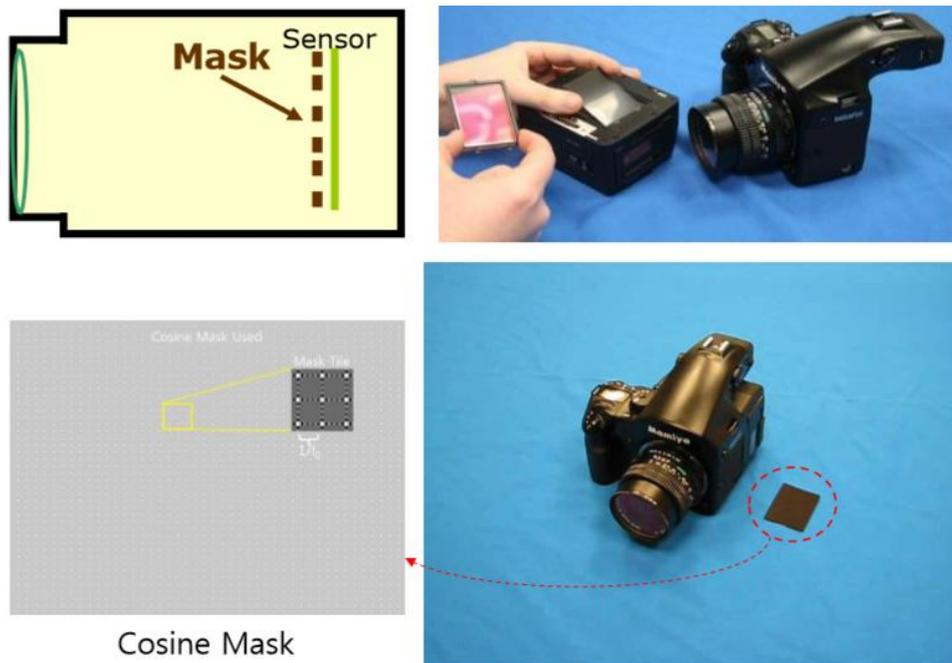
**Gambar 3.18** Kamera light field berbasis mask
