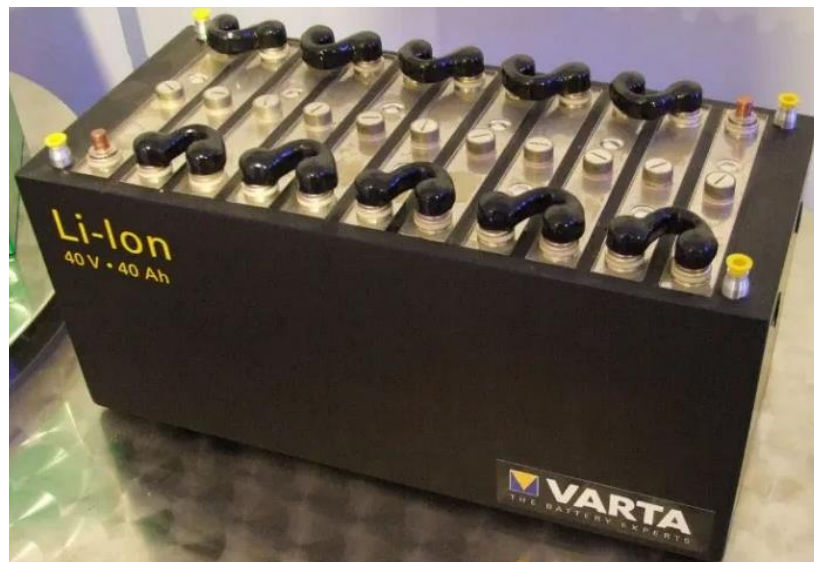
Gambar 8.10 Baterai lithium ion.
