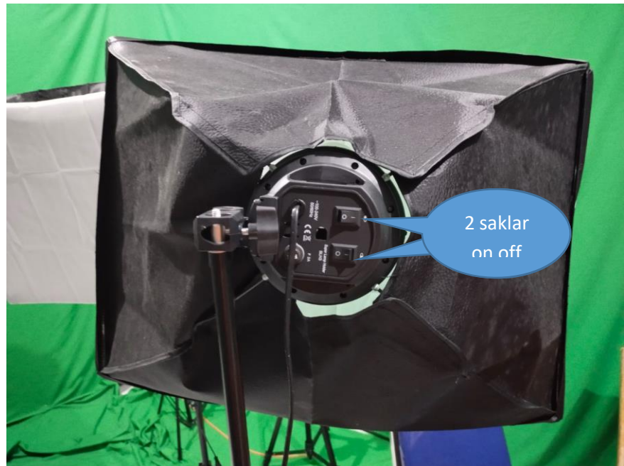
Gambar 10.19 Gambar control power on off lampu softbox 2 saklar
