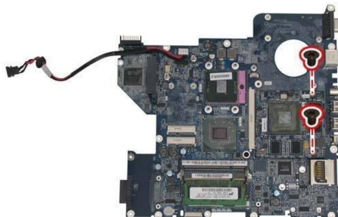
Gambar 4.48 Sekrup VGA Card
