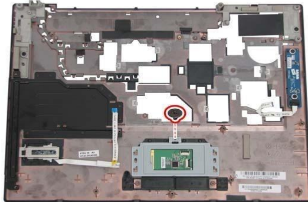
Gambar 5.55 Sekrup Penahan Braket touchpad
