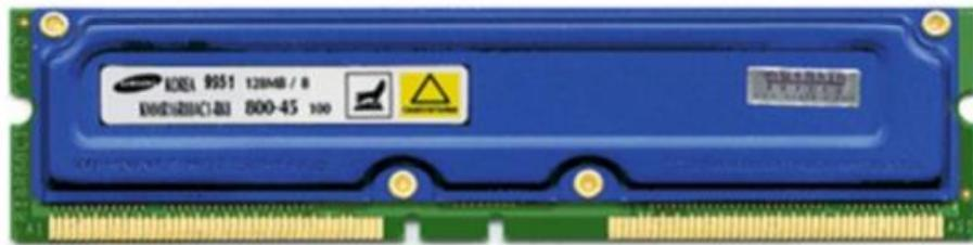
**Gambar 7.5** Modul memori Rambus (Courtesy Samsung Corp.)
