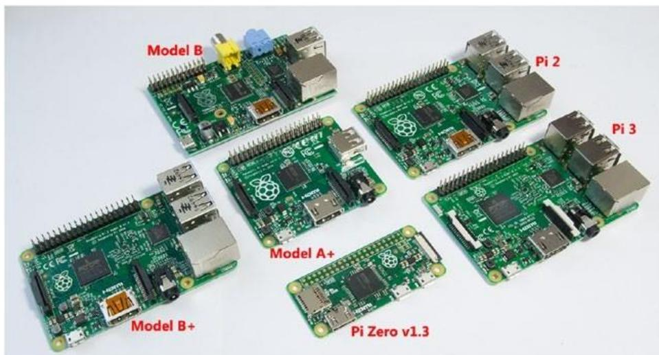
**Gambar 1-1** Raspberry Pi Model B, Model B+, Model A+, Pi 2, Pi 3, dan Pi Zero
