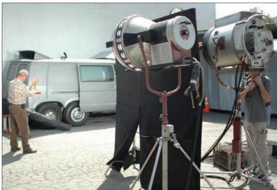
**Gambar 99.** Larry Mole Parker Dari Mole-Richardson Melakukan Uji Berdampingan Dari Lampu Busur Karbon Dan PAR 12K HMI.
