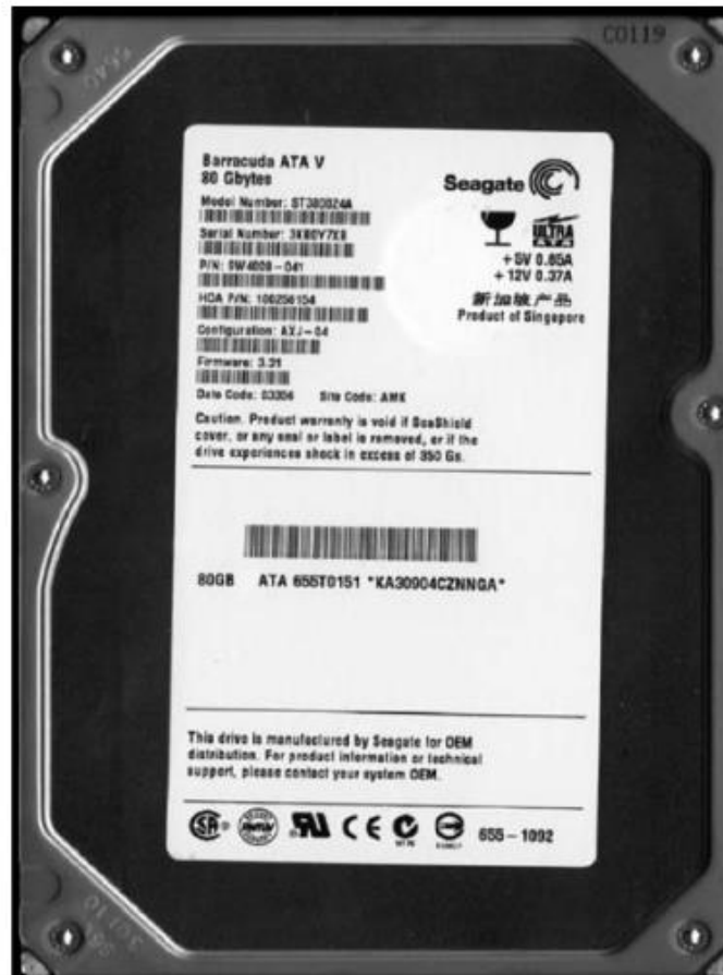
Gambar 10.18 Label Hard Drive
