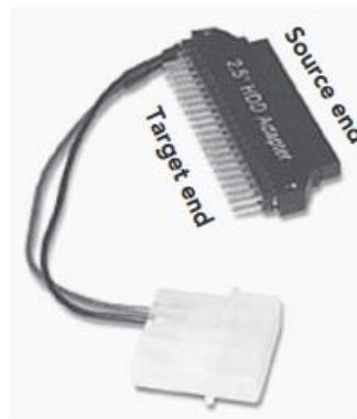
Gambar 10.14 Adaptor Hard Drive Laptop ke IDE
