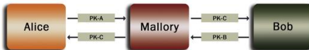
Gambar 4.23 Serangan man-in-the-middle terhadap Diffie-Hellman.
