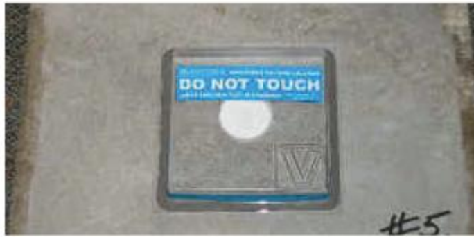
Gambar 6.4 Kit Uji Kalsium Klorida ASTM F1869 dan Meter Kelembaban Relatif ASTM F2170 (Foto milik George Donnelly Testing & Inspections di www.moisturetesting.com ).
