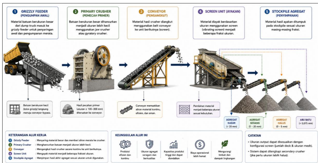
Gambar 9.4 Alur Kerja Stone Crusher Plant
