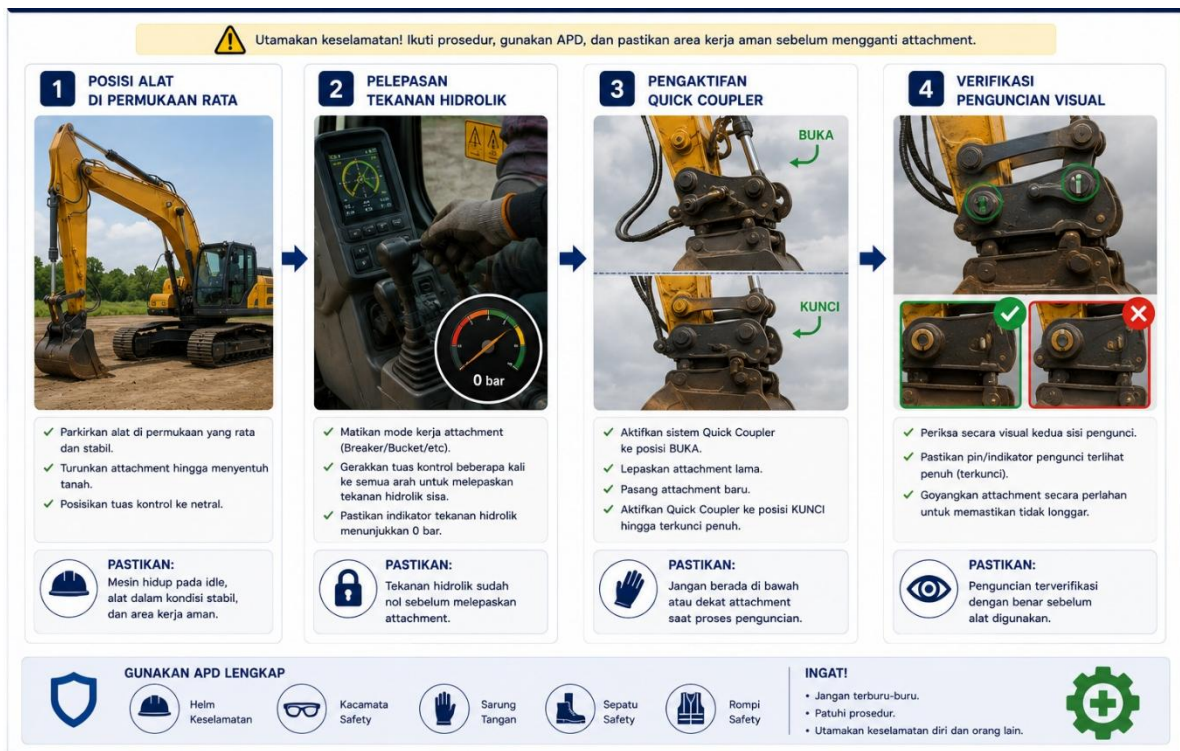
Gambar 10.4 Langkah K3 Penggantian Attachment
