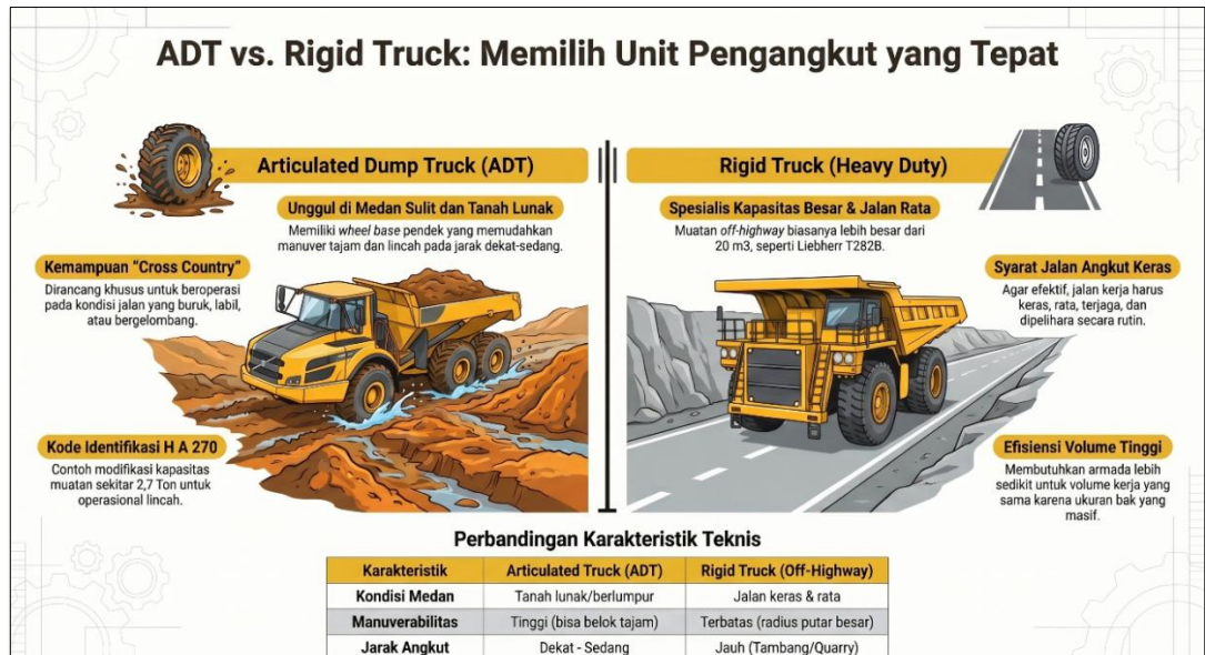
Gambar 6.2 Perbandingan Visual ADT vs. Rigid Truck
