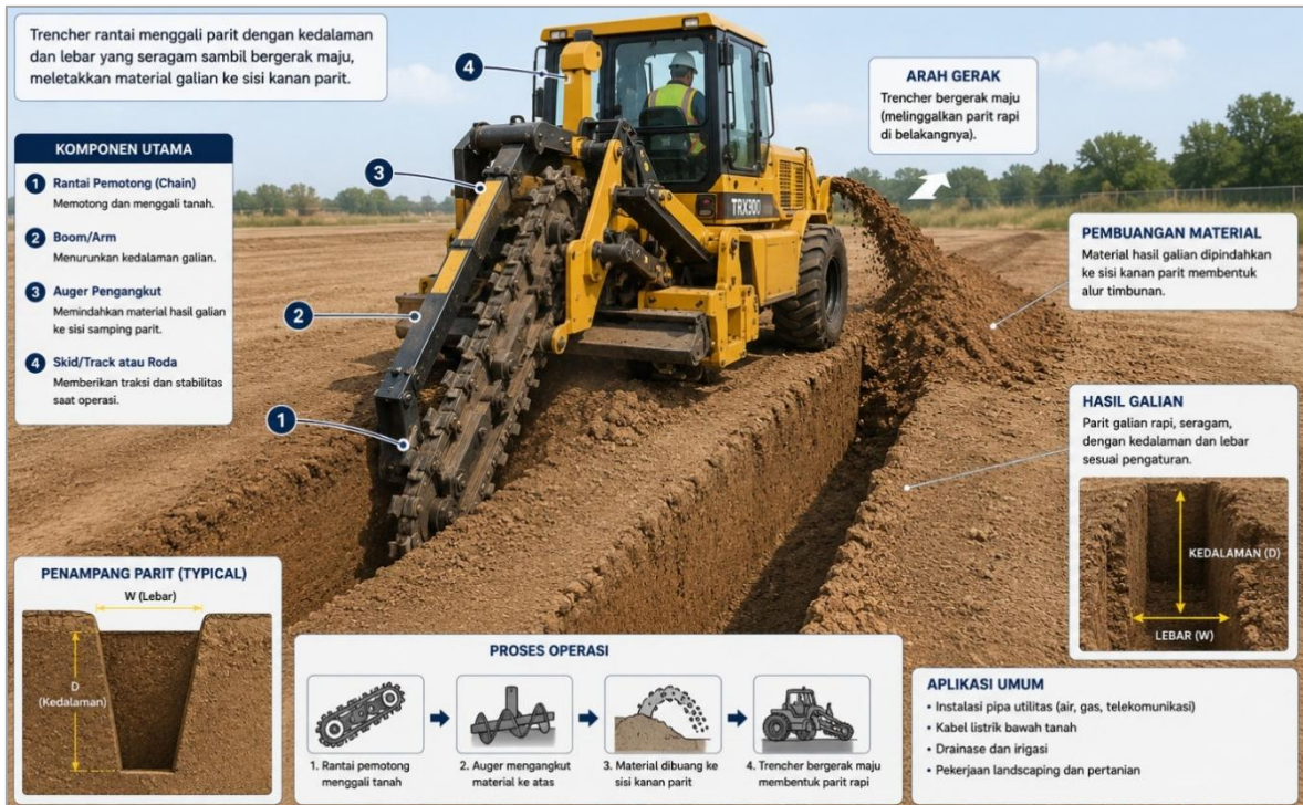
Gambar 9.3 Operasi Trencher Rantai
