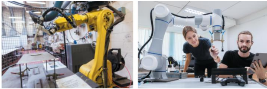
Gambar 5.5 Cobot vs. robot industri tradisional
